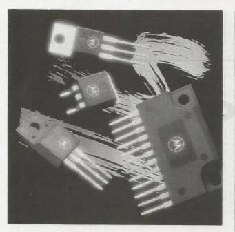
After several years of development, Motorola introduced its first power MOSFETs in 1980. Several technologies were evaluated and the final choice was the double diffused (DMOS) process which Motorola has acronymed TMOS. This process is highly manufacturable and is capable of producing devices with the best characteristics for product needed for power control. Most suppliers of power MOSFETs use the basic DMOS process.
